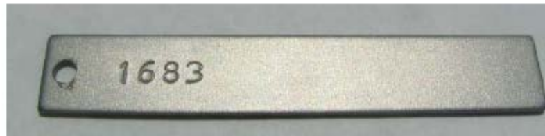
Current Steel Corrosion Rates < 0.1 MPY
