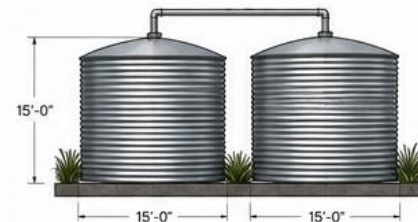
TANK ELEVATION (SIDE YARD)
